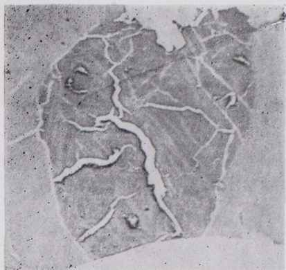
Phot. 1. Electron absorption image of pentlandite containing exsolved lamellae of (\text{Fe, Ni})_1(\text{Co, Ni})_2\text{S}_4 . Magn. \times 460 white — pyroxene, fissures in pentlandite, light-grey — pyrrhotite, dark-grey — pentlandite with light-grey lamellae of (\text{Fe, Ni})_1(\text{Co, Ni})_2\text{S}_4
